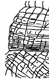
图5 垂直节理系统—多层次组合的龟纹系统(佛陀峰局部) Fig.5 A system of vertical jointing—a system of many-segthence-combined tortoiseshell cracks
