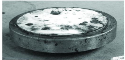
图14 靠近J1的上侧左支座的磨损情况 Fig.14 Abrasion situation of up-left support near J1
