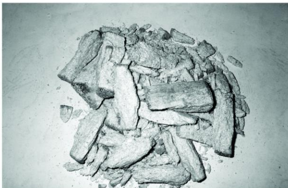
图8 S1撞击后破坏情况 (V=4.79m/s) Fig.8 The fragment after impact loading of S1(V=4.79m/s)
