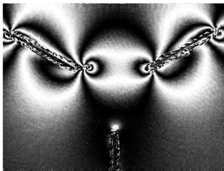
图9 2个45° 的斜裂纹 Fig.9 Two Oblique cracks with 45 degrees
