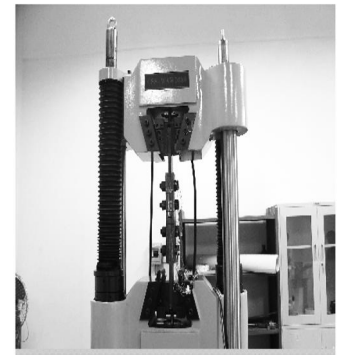
图9 试件拉伸中 Fig.9 Specimen measuring
