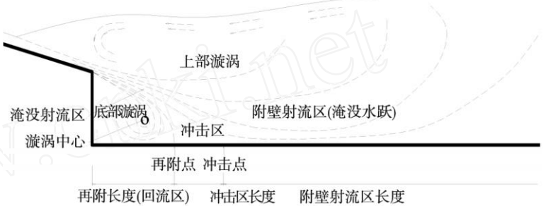
图1 淹没底流流态下消力池内流态示意图 Fig.1 Flow pattern of baffle basin in submerged bottom flow
